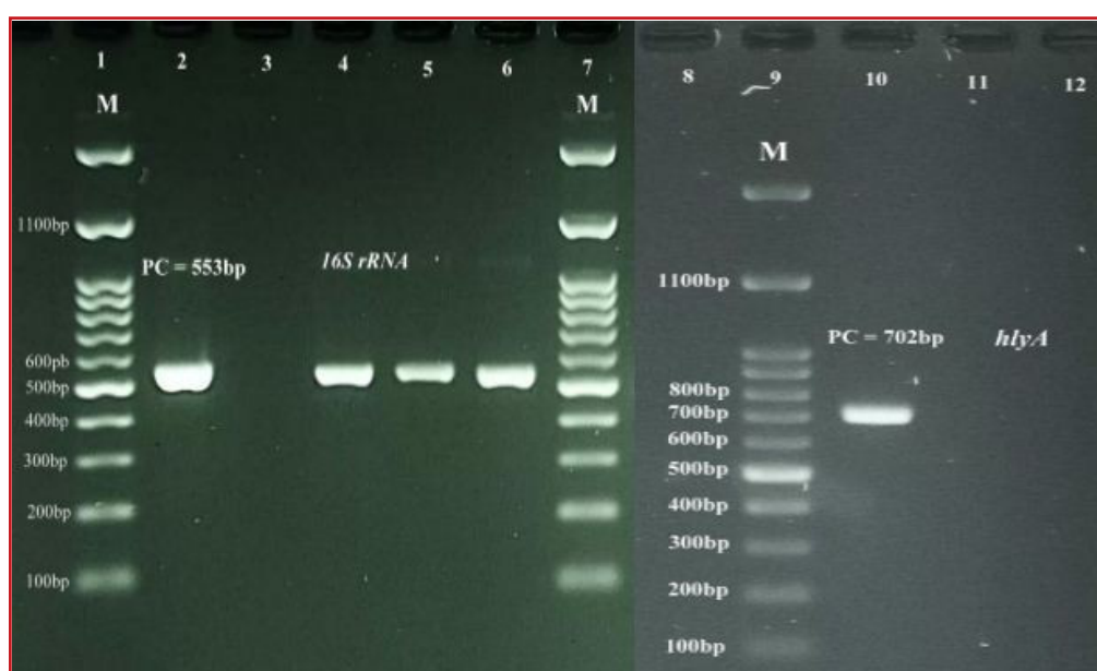
Figure1. PCR assay for the detection of Listeria spp. and L. monocytogenes in raw milk samples. Lane 1, 7, 9 (M) Standard DNA marker; Lane 2: Positive control for Listeria spp; Lane 3: Negative control; Lanes 4–6: Positive samples for Listeria spp; Lane 8: empty; Lane 10: Positive control for L. monocytogenes ; Lane 11: Negative control; Lanes 12: Negative samples for L. monocytogenes . (PC: Positive control)
