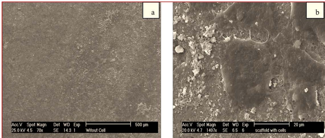
**Figure 3.** SEM micrographs of WJ-MSCs and the shell blocks. Acellular, irregular and nonporous morphology of ventral side of shell (a), WJ-MSCs on the ventral surface of *Cerastoderma lamarcki* (b).
